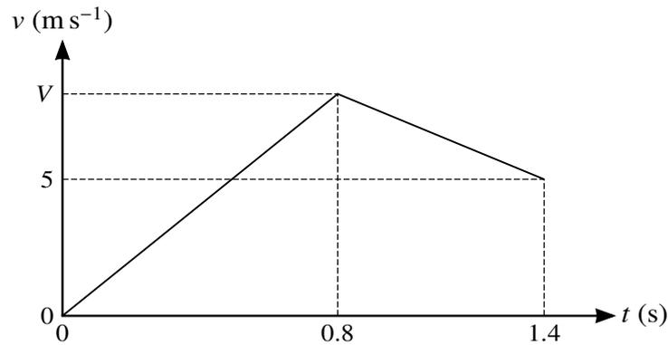
The diagram shows the velocity-time graph for the motion of a small object, which falls vertically from rest at a point  $P$  above the surface of a reservoir. The velocity-time graph consists of two straight line segments.
